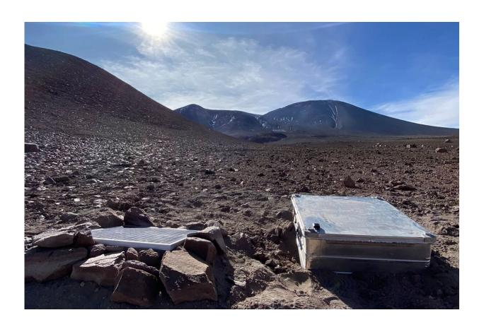
The SO2 camera installation on Lascar Volcano, Chile. The camera is housed inside a protective metal casing, which also holds the battery for powering the instrument; a solar panel for battery charging is located to the left of the box. Credit: Dr Thomas Wilkes
