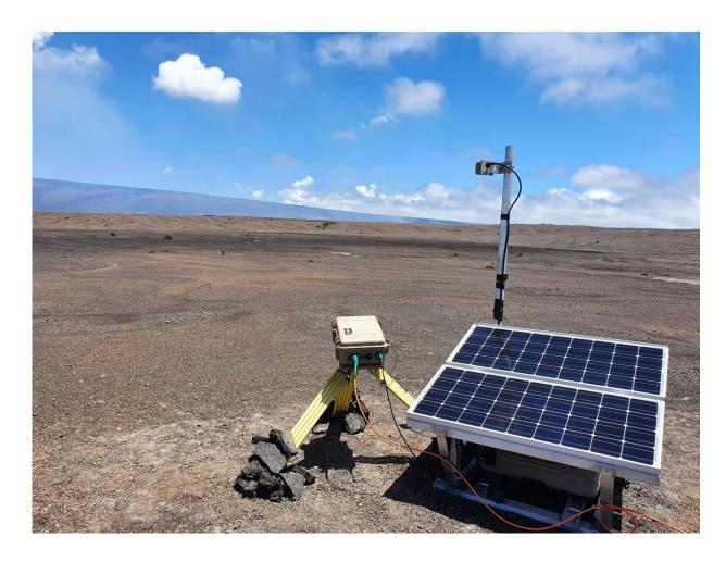
The SO2 camera installation on Kīlauea volcano, Hawaii, US. The gas plume can be faintly seen rising from the crater at the centre of the image and drifting to the left. The flank of Moana Loa can be seen in the background. Credit: Dr Tom Pering
