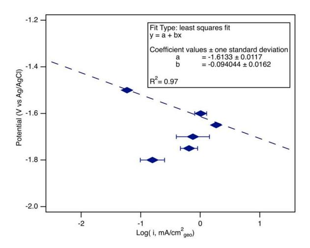
Tafel plot for  $C_2H_4$  corresponding to Figure 1c in the main text. Fit was calculated for first three points on rising edge of volcano (-1.4V to -1.6V) to determine a slope of about 94 mV/dec. Credit: *ACS Catalysis* (2023). DOI: 10.1021/acscatal.2c06043
