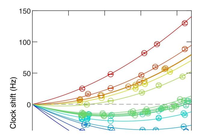
Small shifts of the clock resonance position with the wavelength of the trapping light (color-coded) currently limit the accuracy of the vibrational clock. Credit: K. H. Leung.
