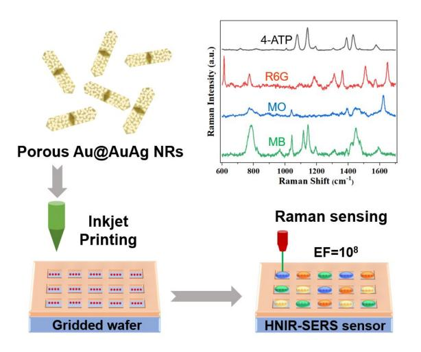
Preparation of the HNIR-SERS sensor and SERS spectra of different molecules with same concentration on the HNIR-SERS sensor. Credit: Wang Yifan
