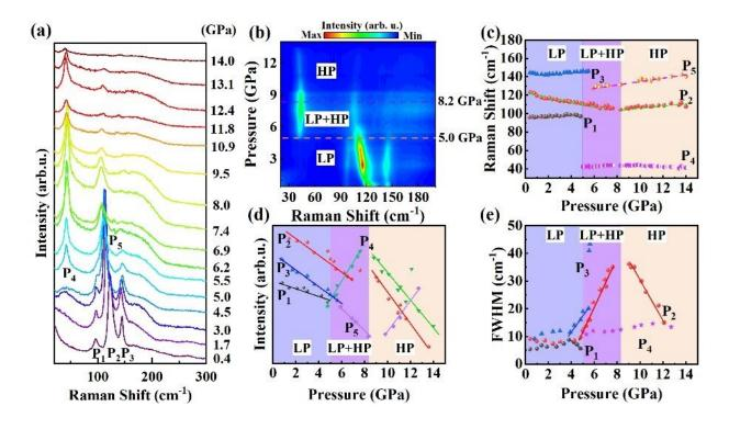
Raman spectra of CrSiTe<sub>3</sub> flakes under pressures up to 14 GPa at room temperature. Credit: Pan Xiaomei
