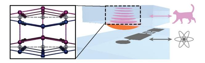
In the ETH Zurich experiment, the cat is represented by oscillations in a crystal (top and blow-up on the left), whereas the decaying atom is emulated by a superconducting circuit (bottom) coupled to the crystal. Credit: ETH Zurich
