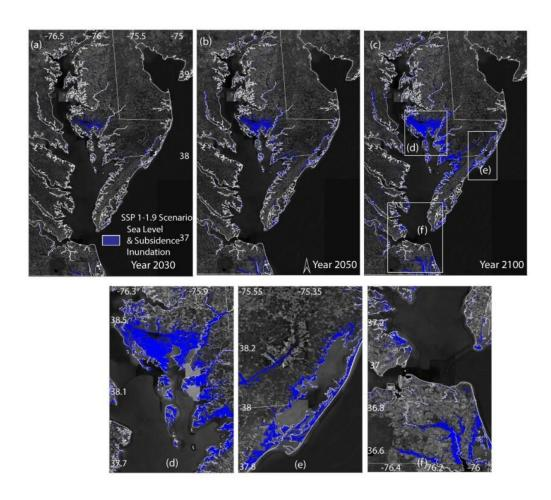
Projected Inundation area from both subsidence and sea level rises under very low greenhouse gases emission scenario at year 2030, 2050, and 2100 (top panels, panels (a), (b), (c), respectively). The bottom panels (d), (e), (f) highlight
