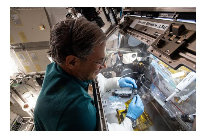
Eytan Stibbe aboard the International Space Station during the Axiom-1 (AX-1) mission in April 2022, shown here with his hands in the life sciences glovebox, or LSG, performing the Fluidic Space Optics experiment of Technion and NASA. During the experiment, Stibbe injected liquid polymers into circular frames to form lenses. He subsequently processed the lenses to harden them for later study on Earth. Credit: Axiom/NASA/Technion
