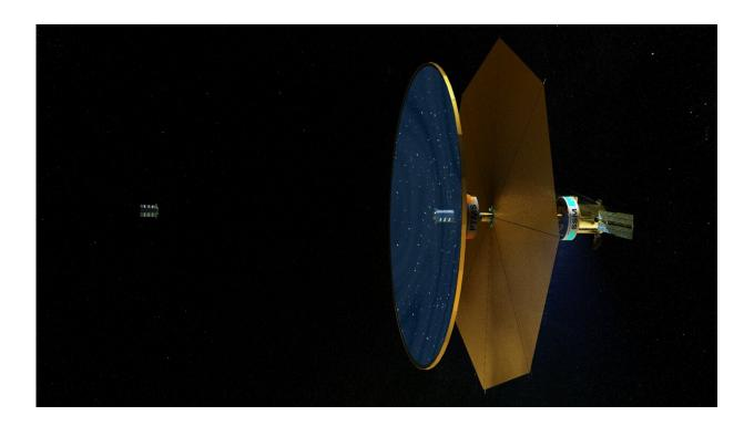
Illustration of the current Fluidic Telescope's (FLUTE's) concept for a next-generation large space observatory. The space telescope's mirror would be created in space from liquid materials and would be approximately 164 feet (50 meters) in diameter – half as long as a football field. The optics would be shaped by the natural surface tension force exerted by fluids. Credits: NASA
