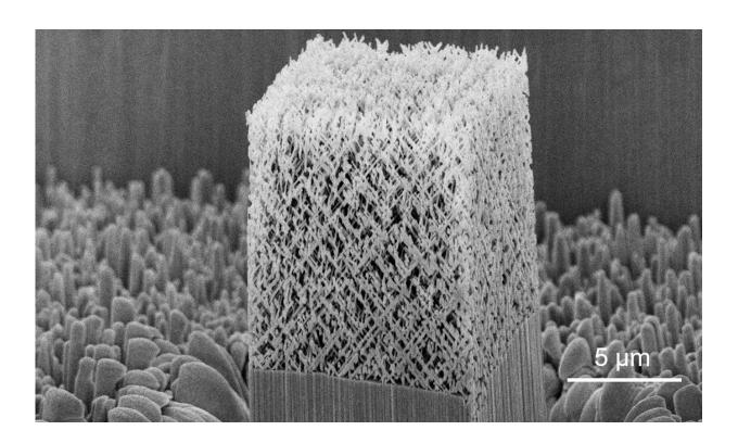
The SEM image of a FIB-milled quasi-BCC beam nanolattice. Credit: IMP
