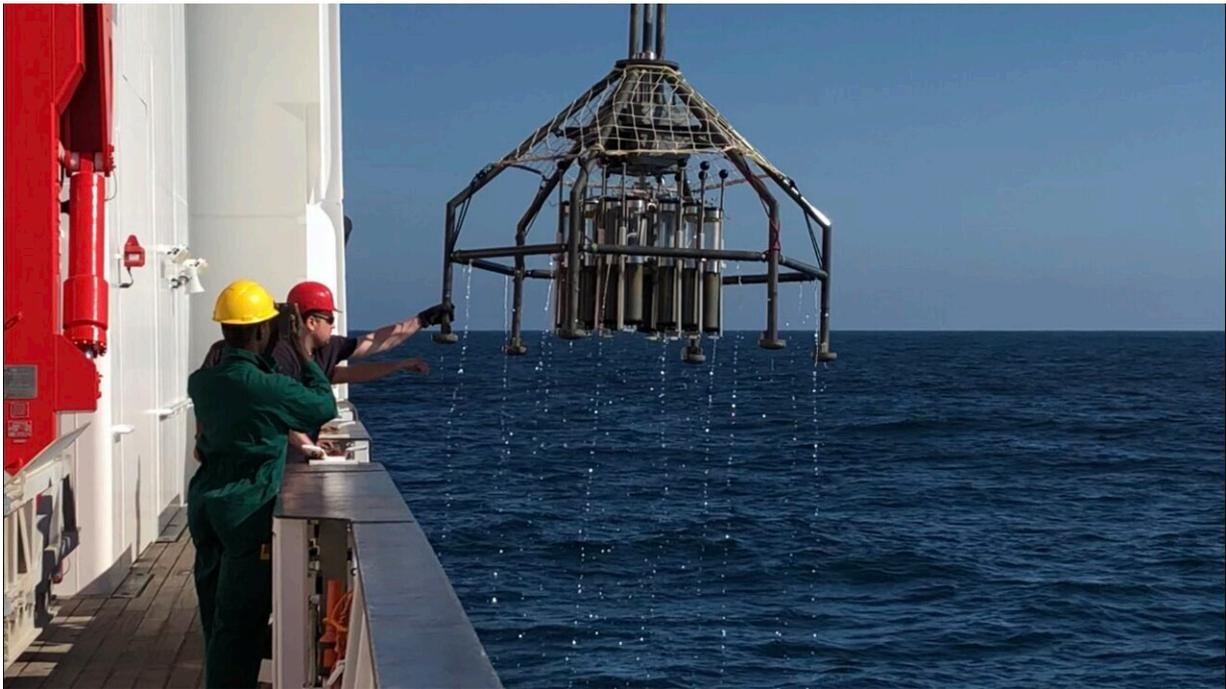
Samples from the bottom of the Atacama trench were taken with this "multiple core sampler", which is shown here on its way up with samples. Credit: Anni Glud/SDU
