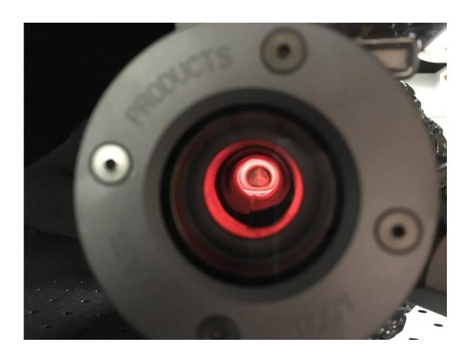
The quantum memory experiment Shinbrough and Lorenz are constructing. It is a cell designed to hold hot metallic vapor, an example of the Lambda-type optical quantum memories that the researchers analyzed. The photograph was taken while the cell was heating, showing molten barium at the bottom before it
