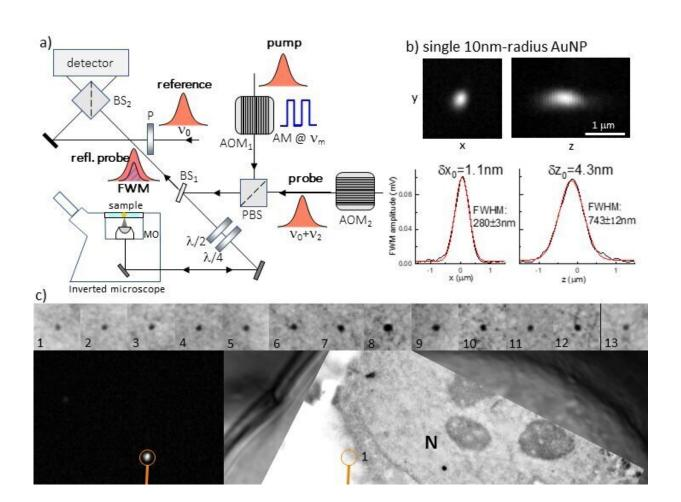
a) Sketch of FWM set-up. Short optical pulses in resonance with the optical absorption peak of a gold nanoparticle (AuNP) are focused onto the sample, using an inverted microscope, and generate a FWM field which is collected in epi-geometry, detected with a heterodyne interference scheme. AOM: acousto-optic modulator. (P)BS: (polarising) beam splitter. P: polariser. MO: microscope objective. b) Example of volumetric FWM microscopy on a single 10nm-radius
