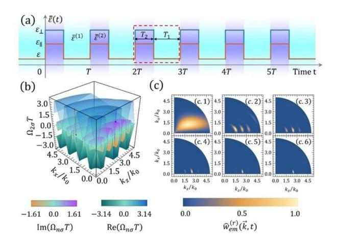
(a) Schematic of the APTC; (b) Band structure of the APTC; (c) Normalized radiative energy in momentum space at various time instants of the APTC due to an embedded stationary charge. Credit: *Physical Review Letters* (2023). DOI: 10.1103/PhysRevLett.130.093803
