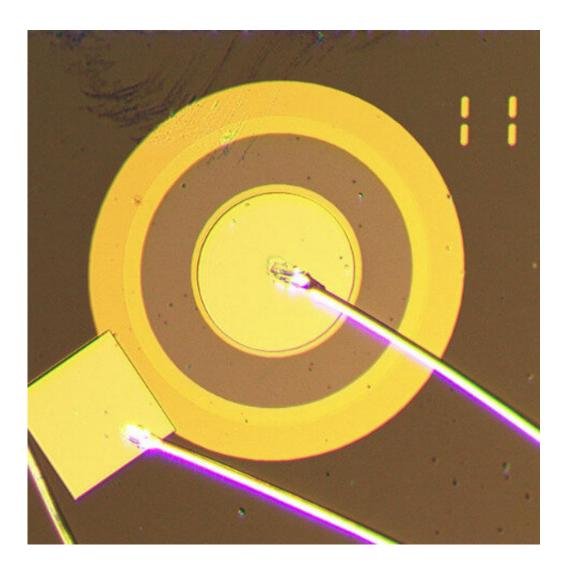
The donut-like structure of the device used in experiments demonstrating Laughlin charge pumping in an edge-free device. Credit: RIKEN Center for Emergent Matter Science
