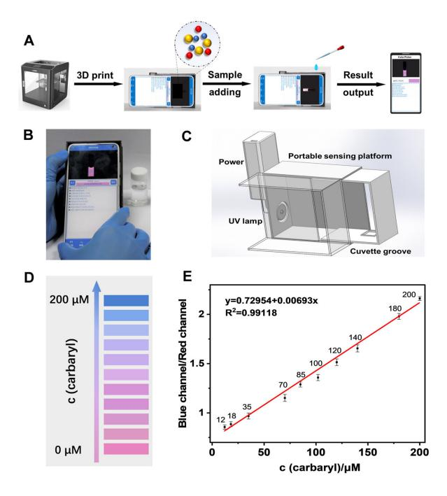
Schematic diagram of a smartphone sensing platform detecting carbaryl. Credit: Zhang Zhong
