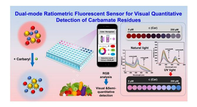
Schematic diagram of a dual-modal sensor for rapid visualization and quantitative detection of carbaryl residues. Credit: Zhang Zhong
