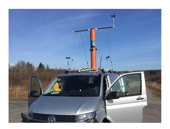
To make the measurements, a car was used to move a model of a shouter, generating wind past it. Credit: Aalto University
