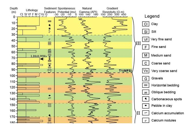
Lithology, sample locations, log curves and sedimentary facies classification of the borehole in the deposition center of the Banquan basin. Credit: Science China Press
