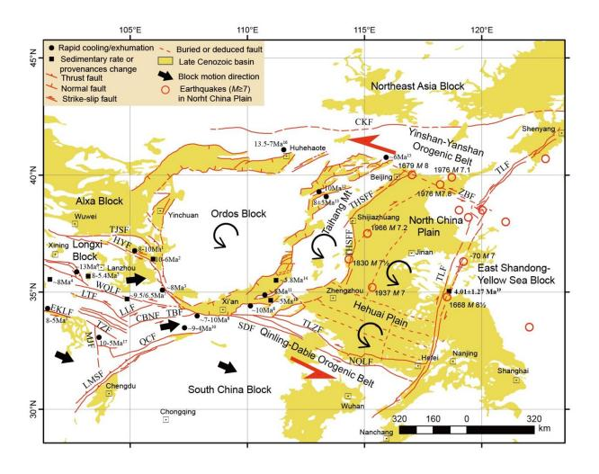
The faults and their properties are based on Deng et al. (2007) and Xu et al. (2016); fault architecture in the North China Plain is mainly according to Yin et al. (2015), Xu et al. (2019) and Zhang et al. (2019); main fault abbreviations are as follows: EKLF-East Kunlun fault, TZF-Ta Zang fault, MJF-Min Jiang fault, LMSF-Longmenshan fault; QCF-Qing Chuan fault, LDF-Lintan-Dangcang fault, LLF-Lixian-Luojiabao fault, CBNF-Chengxian Basin Northern fault, TBF-
