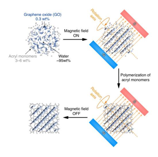
Schematic illustration for the preparation of the composite hydrogel withunidirectionally aligned GO nanosheets. Credit: *Science* (2023). DOI: 10.1126/science.adf1206
