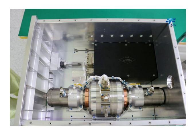
The uncapped Stirling thermoelectric converter. Credit: China Manned Space Agency
