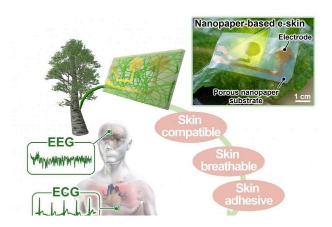
Schematic of the nanopaper-based e-skin for harmonious on-skin monitoring of Electroencephalogram (EEG), electrocardiogram (ECG), and electromyogram (EMG). Credit: Huang et al, *Advanced Materials Interfaces*, CC BY
