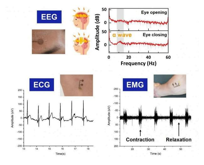
On-skin EEG, ECG, and EMG signals acquired by attaching the nanopaperbased e-skin on the human skin surface. Credit: Huang et al, *Advanced Materials Interfaces*, CC BY
