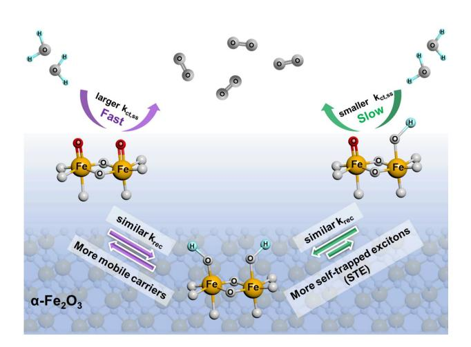
The UV irradiation reduces the formation probability of self-trapped excitons and significantly promotes the multi-hole accumulation process, thereby achieving the efficient water oxidation reaction even under low bias. Credit: Science China Press
