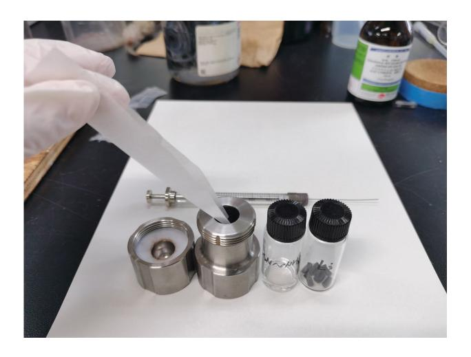
Ball milling jar and reagents used in the simplified mechanochemical Birch reduction. Credit: Koji Kubota
