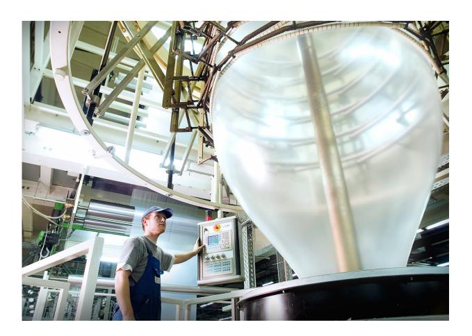
The bioplastic films made from PBS developed as part of the RUBIO project are recyclable, biodegradable and can be processed on standard extrusion lines. Credit: POLIFILM
