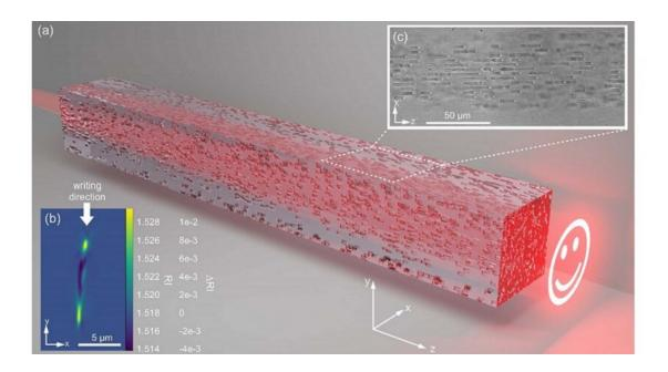
The intensity shaper can convert an input Gaussian beam to precisely direct light, as in (a) "smiley" light distribution. Precision arrangement of voxels is achieved using ultrafast direct laser writing. (c) Each voxel is a micron-sized element with (b) a specific refractive index profile along the x and y axes. Credit: Barré et al., doi 10.1117/1.APN.2.3.036006.
