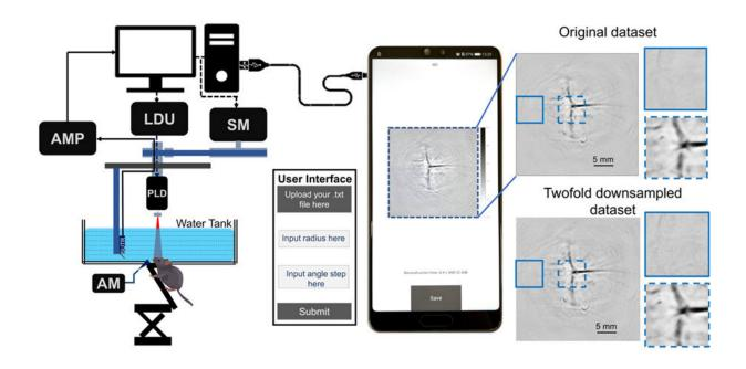
Experimental pulsed laser diode based in vivo PAT imaging system. Reconstructed PAT images, displayed on the Android mobile platform-based application. In vivo PAT reconstructed rat brain vasculature image with original dataset and twofold downsampled dataset. Credit: Hui et al., doi 10.1117/1.JBO.28.4.046009
