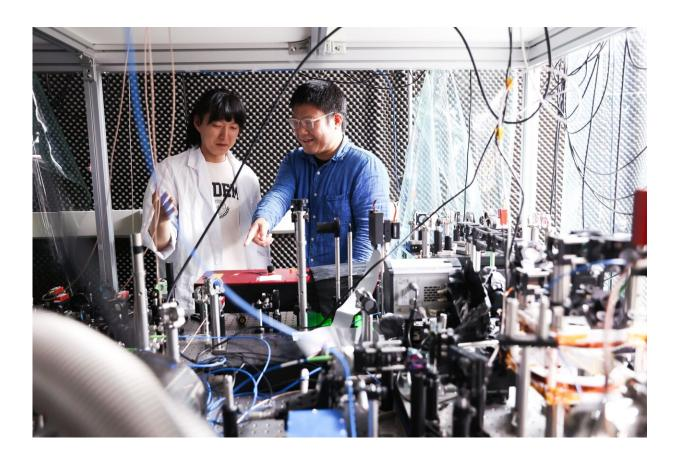
Research team members Hansub Hwang (left) and Andrew Byun (right) are pictured with the optical setup used to create free-flying atoms. For throwing, a trap holding an atom is accelerated and then turned off, which causes the atom to launch out of the trap. Another trap is then turned on to capture the incoming atom and decelerated until the atom stops completely. Credit: Jaewook Ahn, Korea Advanced Institute of Science and Technology
