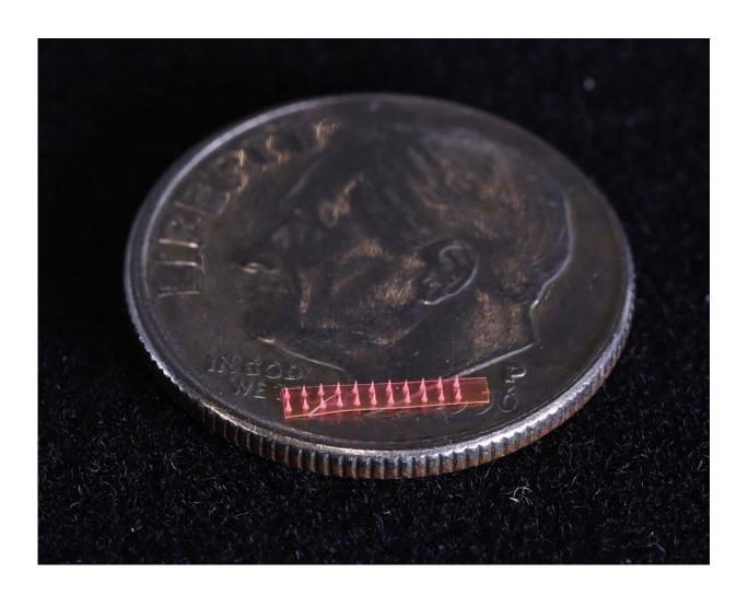
Illustration of a silk microneedle array on a dime coin. Credit: Singapore-MIT Alliance for Research and Technology (SMART)
