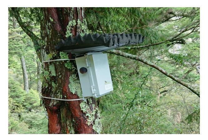
An automatic recorder was installed on a tree to capture the surrounding soundscape. Credit: Ph.D. Candidate Shih-Hung Wu
