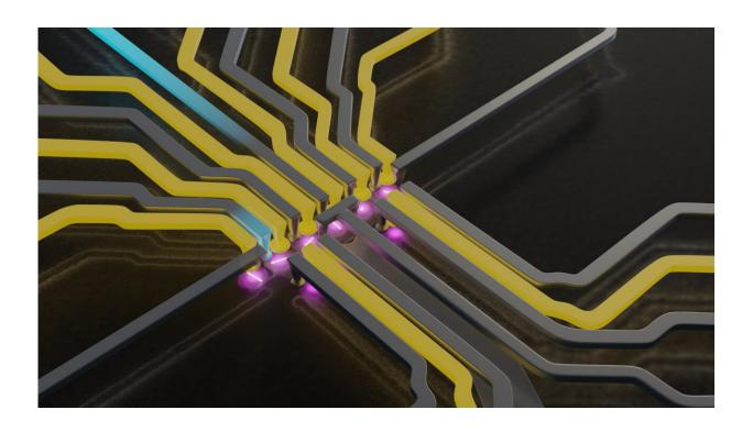
Render of a six-dot SLEDGE device in silicon, which implemented universal logic with encoded spin qubits. Credit: HRL Laboratories
