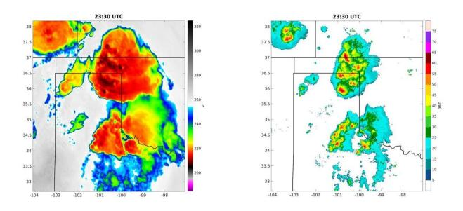
The first figure (left) shows satellite brightness temperatures when thunderstorms developed and matured in the case study, and the second shows a radar image of the same storms at the same time. The scientists said combining the data in weather models may improve forecasts. Credit: Penn State
