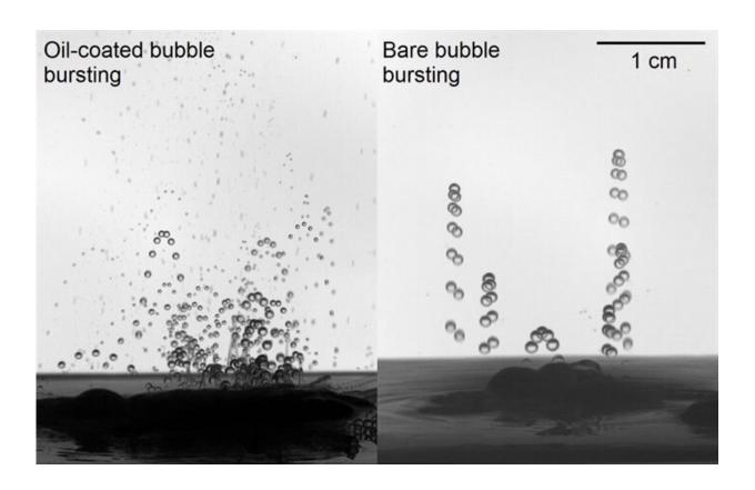
Oil-coated bubble bursting (left) compared to bare bubble bursting (right.). Credit: The Grainger College of Engineering at University of Illinois Urbana-Champaign
