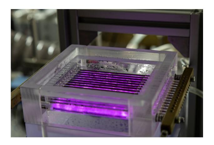
Plasma in water spray: A contaminated water sample is nebulised via a nozzle and sprayed into a dielectric barrier discharge, which is ignited between two layers of metal and ceramic rods. Credit: INP
