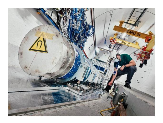
The FASER particle detector, located deep underground at CERN's Large Hadron Collider, was mostly built out of spare parts from other experiments at CERN. Credit: CERN
