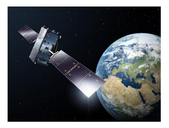
Galileo satellites are placed in medium orbits, at 23 222 km altitude along three orbital planes so that a minimum of four satellites will be visible to user receivers at any point on Earth once the constellation is complete. The fifth and sixth Galileo satellites, launched together on 22 August 2014, ended up in an elongated orbit travelling out to 25 900 km above Earth and back down to 13 713 km. In addition, the orbits are angled relative to the equator less than
