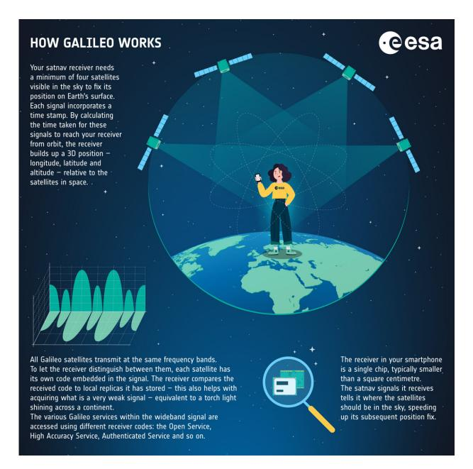
Your satnav receiver needs a minimum of four satellites visible in the sky to fix its position on Earth's surface. Each signal incorporates a time stamp. By calculating the time taken for these signals to reach your receiver from orbit, the receiver builds up a 3D position—longitude, latitude and altitude—relative to the satellites in space. Credit: European Space Agency
