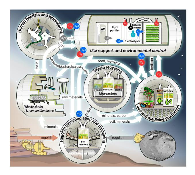
Graphical rendering of a microbial biotechnology-based life-support system in an agnostic space environment. Microorganisms are included in all the functional
