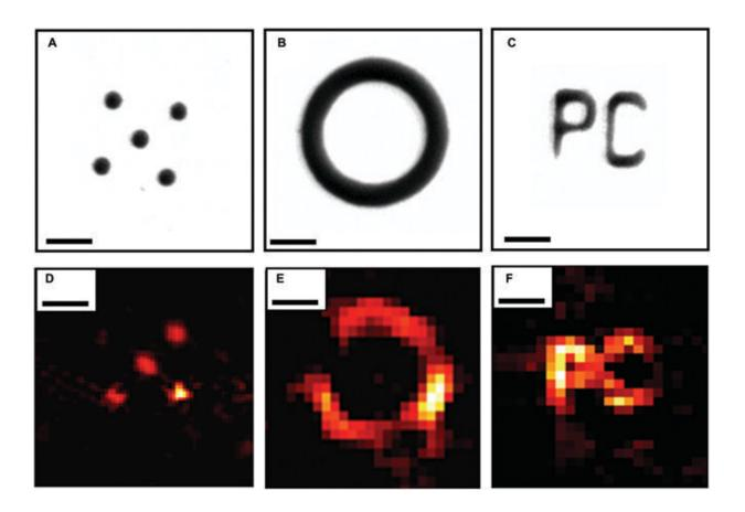
(A to C) Photographs of three samples obtained with a conventional transmission microscope. (D to F) Corresponding objects reconstructed from photoacoustic measurements obtained by scanning unknown speckle patterns over the sample hidden behind a diffuser, with use of the optical memory effect. Scale bars, 25 micrometers. Images D to F are believed to be the first obtained in such a manner. Credit: Antonio M. Caravaca-Aguirre et al.
