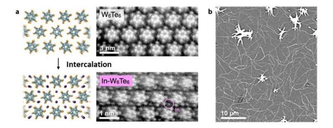
(a) Schematic of atomic structure of both tungsten telluride nanofiber bundles and the final intercalated structure, along with scanning transmission electron microscopy images. (b) Synthesized 3D TMC nanofibers on a silicon substrate. Credit: Tokyo Metropolitan University
