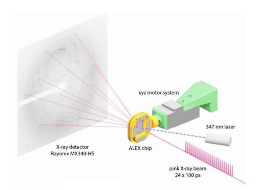
This schematic shows the experimental setup for serial crystallography, which uses a nylon chip containing tens of thousands of protein crystals that can be quickly scanned with an X-ray beam. Credit: Argonne/Andrzej Joachimiak
