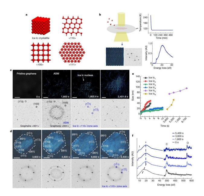
Observation of cubic ice formation on graphene at 102 K by in situ cryogenic TEM. Credit: Institute of Physics
