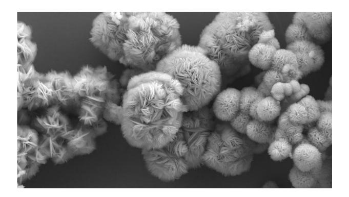
A scanning electron microscopy image reveals the beautiful shapes of tiny structures known as MXenes, which are of interest to scientists for new devices and electronics but were previously hard to create. These were grown with a new easier and less toxic method invented by chemists with the University of Chicago. For reference, the diameter of a human hair is about 50  $\mu$ m. Credit: Di Wang
