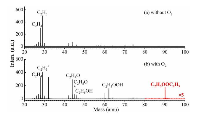
VUV lamp photoionization mass spectra measured (a) without  $O_2$  and (b) with  $O_2$  in the microwave discharge flow tube, with five times magnified data in red. Credit: Lin Xiaoxiao
