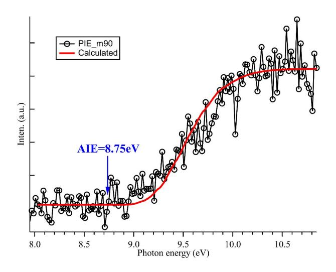
Photoionization spectrum of  $C_2H_5OOC_2H_5$  and its calculated results in red. Credit: Xiaoxiao
