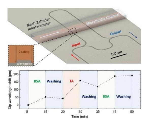
Working principle of the hybrid photonic-microfluidic chip in the example of a Mach-Zehnder interferometer. Credit: Skolkovo Institute of Science and Technology
