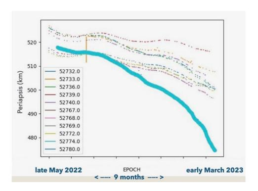
The graph shows how much lower SBUDNIC's orbit, represented by the thick blue line, is compared with other devices deployed with it from late May 2022 to early March 2023. Credit: Brown University
