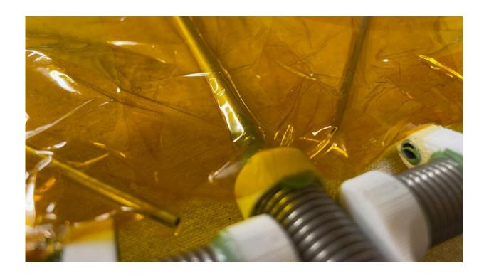
The Kapton polyimide drag sail, attached to the SBUDNIC satellite, is helping to push the satellite back down to Earth sooner. Credit: Marco Cross
