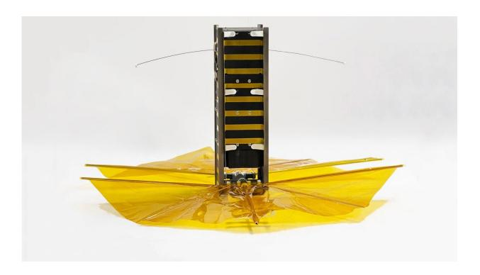
SBUDNIC, a bread-loaf-sized cube satellite with a drag sail made from Kapton polyimide film, designed and built by students at Brown was launched into space last May on a SpaceX rocket. Credit: Marco Cross
