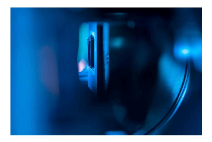
View inside the vacuum chamber, where we trap strontium and calcium ions using electric fields and lasers. Credits: David Nadlinger.
