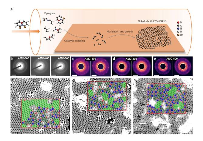
a. Schematic diagram of AMC growth mechanism; b-h. Atomic-scale structural characterizations of AMC. Credit: Liu Lei
