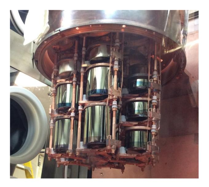
The inner detector arrangement. The silver cylinders are the Ge detectors. They are contained within a vacuum chamber and the outer wall of that chamber is not in place in this figure. Credit: Majorana Collaboration.
