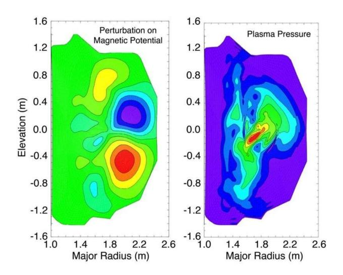
DIII-D plasma simulation during thermal quench shows structures of magnetic perturbation and pressure due to the instability. Color indicates relative value, showing that plasma instability generates a pressure profile expelling particles to the wall. Credit: *Physics of Plasmas* (2022). DOI: 10.1063/5.0107048
