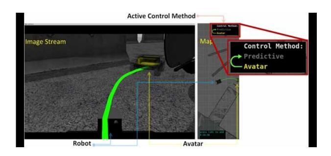
Hybrid teleoperation interface (adjustable autonomy) to cope with latency conditions - augmented interface allows to switch between two control methods: (1) direct control with predictive elements and (2) semi-autonomous control resorting to virtual element (avatar). Credit: *IEEE Access* (2023). DOI: 10.1109/ACCESS.2023.3240307
