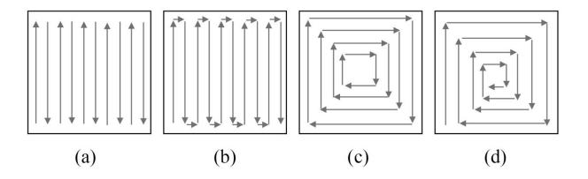
Common toolpath patterns used in additive manufacturing technologies: a) raster, b) zigzag, c) contour, and d) spiral. Credit: Ezgi Pulatsu and Chibuike Udenigwe
