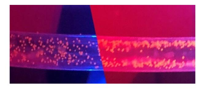
Microplastics naturally scatter in flowing water (left), but after turning on sound waves, the particles concentrate along the tube's sides (right), making them easier to remove. Credit: Menake Piyasena
